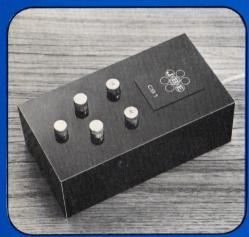
The transformer is also situated in the control box thus minimising interference to tone arm and stylus
